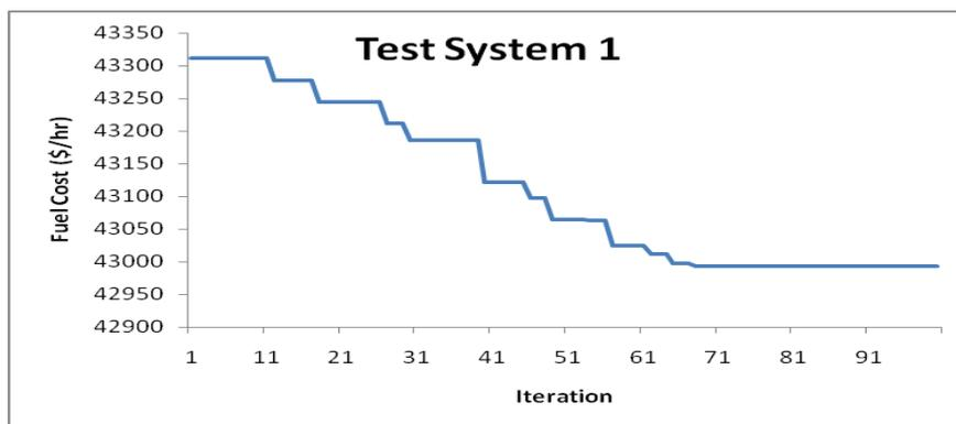
Fig. 2 Convergence curve of the Test system 1
